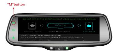
2: Using iPhone search WIFI (WIFI name is displayed on the screen and shown as below), then enter the default password::12345678. After finishing WIFI connection, bring up the shortcut menu, click on the AirPlay function, select the device name, and open the Mirroring.
